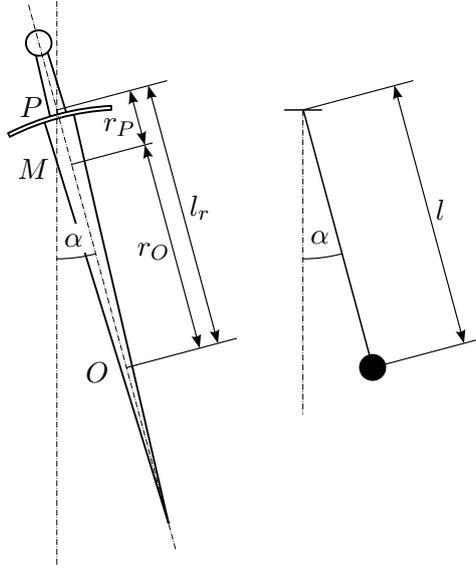
Figure 1: The sword as a physical pendulum and a mathematical pendulum with the same angular eigenfrequency  $\omega_0$
